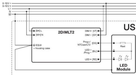
494749\_Wiring Diagramm 2DIMLT2 with LEDset2
