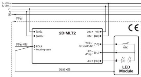
494748\_Wiring Diagramm 2DIMLT2 with NTC
